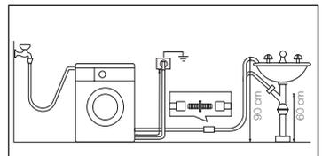
For the correct functioning of the machine, the drain hose must remain hooked on the proper support piece situated on the top part of back side of the appliance.
