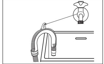
In this case, make sure the end cannot come unhooked when the machine will be emptied.
