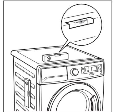
If you do not have a spirit level, as a guide use the edge of a door frame, cupboard or bench to check that the washer-dryer is leveled.
