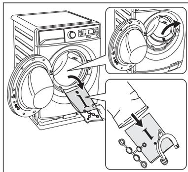
4. Put one of the polystyrene packaging elements on the floor behind the appliance. Carefully put down the appliance with the rear side on it. Make sure not to damage the hoses.
