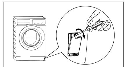
3. Pull **twice** the emergency unlock trigger downward then open the appliance door.
