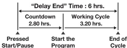
After select Delay End time, press Start/Pause touchpad to start the program. Machine will then countdown and update time on the display every hours until it reaches the starting point of the wash cycle.
