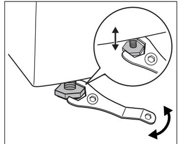
When the washing machine is levelled, try to rock it from corner to corner. If it does rock, adjust the legs again until it is levelled and does not rock.
