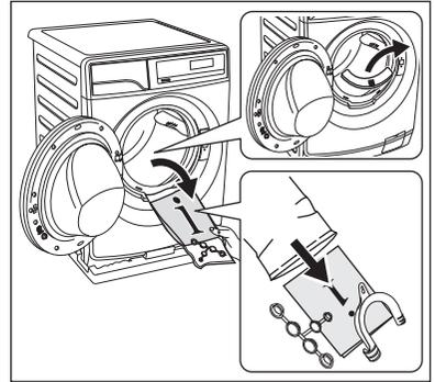
4. Put one of the polystyrene packaging elements on the floor behind the appliance. Carefully put down the appliance with the rear side on it. Make sure not to damage the hoses.
