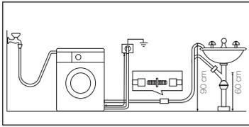
For the correct functioning of the machine, the drain hose must remain hooked on the proper support piece situated on the top part of back side of the appliance.
