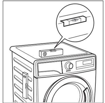
If you do not have a spirit level, as a guide use the edge of a door frame, cupboard or bench to check that the washing machine is leveled.
