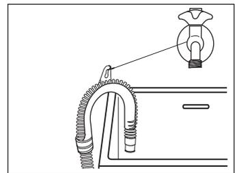
In this case, make sure the end cannot come unhooked when the machine will be emptied.
