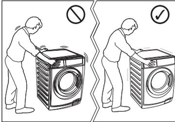
Never place cardboard, wood or similar materials under the machine to compensate for any unevenness in the floor. Install the machine on a flat hard floor. Make sure that air circulation around the machine is not impeded by carpets, rugs etc.
