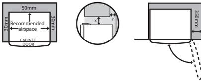
If you have a cupboard above the refrigerator with a rear gap of less than 100 mm (Y), recommended clearance at the top of the refrigerator increases from 50mm to 90mm (X) minimum.
