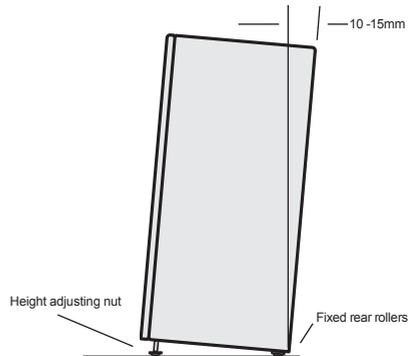
3. Wind the large height adjusting nut on the handle side down until the refrigerator is level and stable. If you have difficulty winding the nut or height adjusting foot down, have someone tilt the refrigerator back so you have better access.
