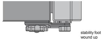
4. Check the alignment of the refrigerator to the surrounding cupboards to see if it is level. You can adjust the level as detailed in step 2 and 3.
