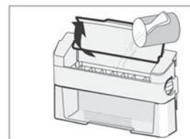
After the water completely freezes, turn the knob clockwise, ice cubes will fall down into the ice container. It takes about 3 hours for water to completely freeze if the water is 20°C when filled.
