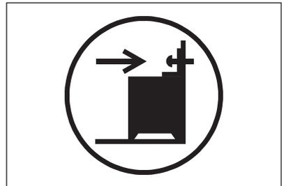
1. Install the anti-tilt protection 232 - 237 mm down from the top surface of the appliance and 110 - 115 mm from the side of the appliance into the circular hole on a bracket. Screw it into the solid material or use applicable reinforcement (wall).
