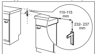
2. You can find the hole on the left side at the back of the appliance. Lift the front of the appliance and put it in the middle of the space between the cupboards. If the space between the bench cupboards is larger than the width of the appliance, you must adjust the side measurement to centre the appliance.
